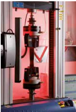
PELSTERKTE OVERLAP - Dynamometer. Standard UNI EN 12316-1.
