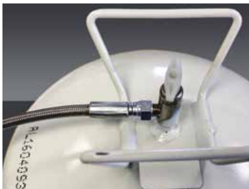
Image 1 - Canister with the braided-hose attached properly.
